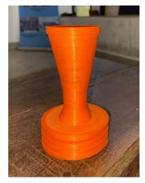
The students utilized 3D printers to produce an innovative rocket nozzle. The intricate and precise manufacturing process enables the creation of complex nozzle geometries, optimizing the flow of propellants and combustion gases. As a result, it improves the rocket's overall performance and reliability
